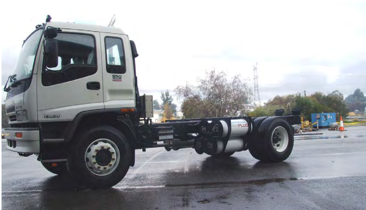
Figure 3.46 New dedicated SI CNG truck with fuel storage for about 200 km 17
